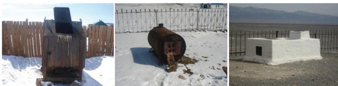
Photo 2. Incinerators for medical waste in rural area
